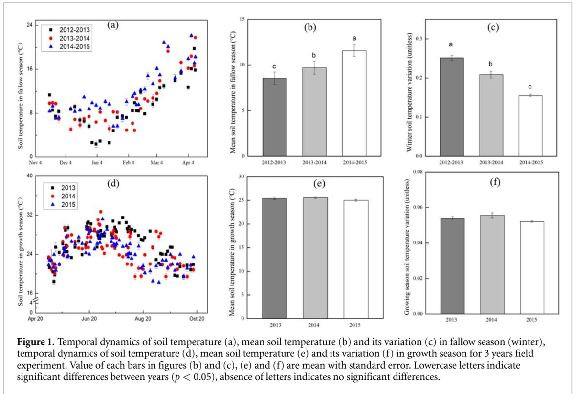
**Figure 1.** Temporal dynamics of soil temperature (a), mean soil temperature (b) and its variation (c) in fallow season (winter), temporal dynamics of soil temperature (d), mean soil temperature (e) and its variation (f) in growth season for 3 years field experiment. Value of each bars in figures (b) and (c), (e) and (f) are mean with standard error. Lowercase letters indicate significant differences between years ( $p < 0.05$ ), absence of letters indicates no significant differences.
