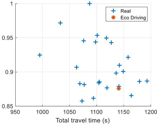
**Figure 5: Normalized battery energy consumption according to the total travel time**
