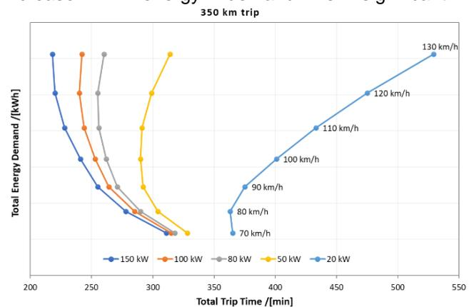
**Figure 1: Dependency between available charging power, energy demand and trip time for a long distance trip**
