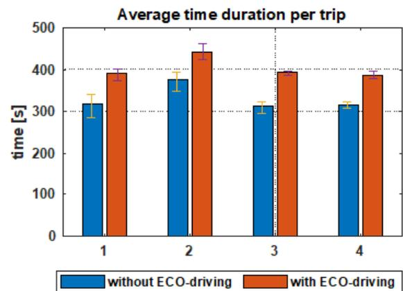
**Figure 15: Trip duration with and without ECO-driving for the two directions of the trip**
