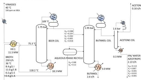
Fig 2. Flowsheet of the 3 columns base case
