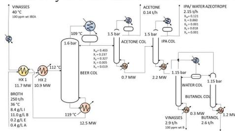
Fig 1. Flowsheet of the 5 columns reference case
