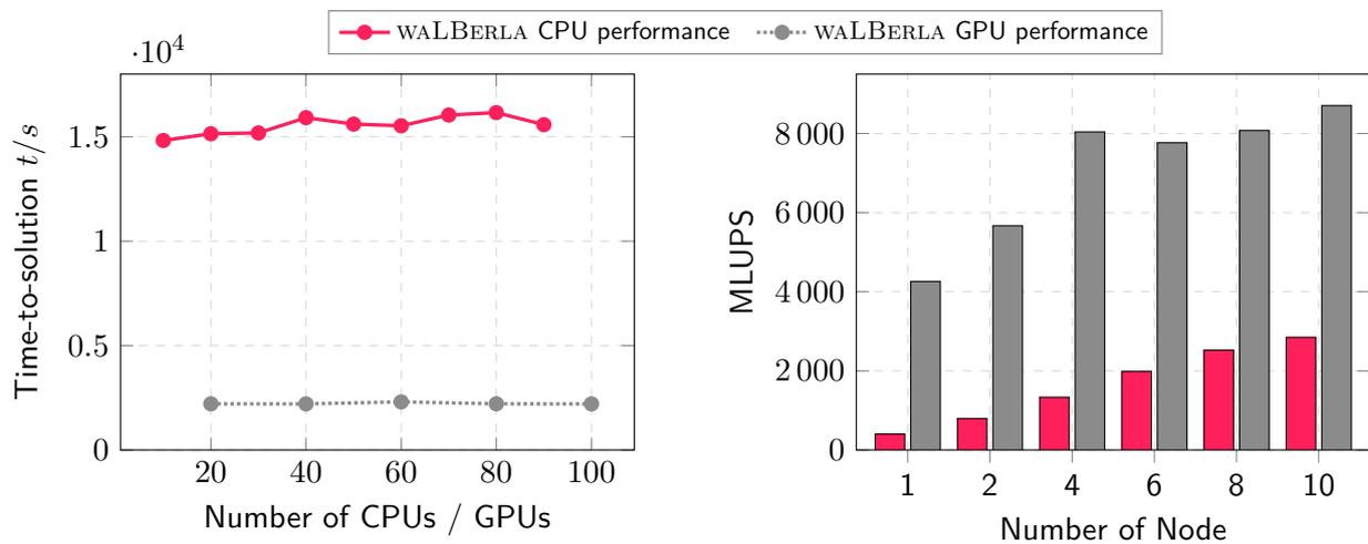
**Figure 4.** WALBERLA scaling experiments for 1 200s simulated physical time with  $\Delta t = 0.010054s$ : weak scaling with 40 960 000 cells per node (left), strong scaling with 163 840 000 cells (right)
