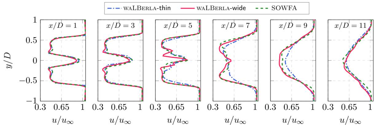
**Figure 2.** Wake velocity profiles, 64 cells per diameter
