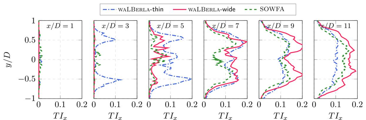
**Figure 3.** Wake TI profiles, 64 cells per diameter
