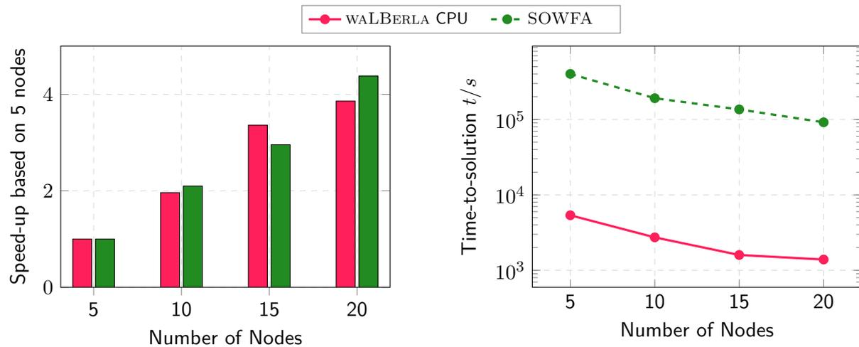
**Figure 5.** Strong scaling experiment with 163 840 000 cells, 1 200s simulated physical time with  $\Delta t = 0.026s$ : Speed-up based on the simulation time on five nodes (left), performance in time-to-solution (right)
