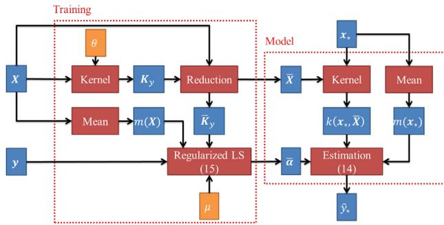
Fig. 1. Schematic of the algorithm for one cluster.
