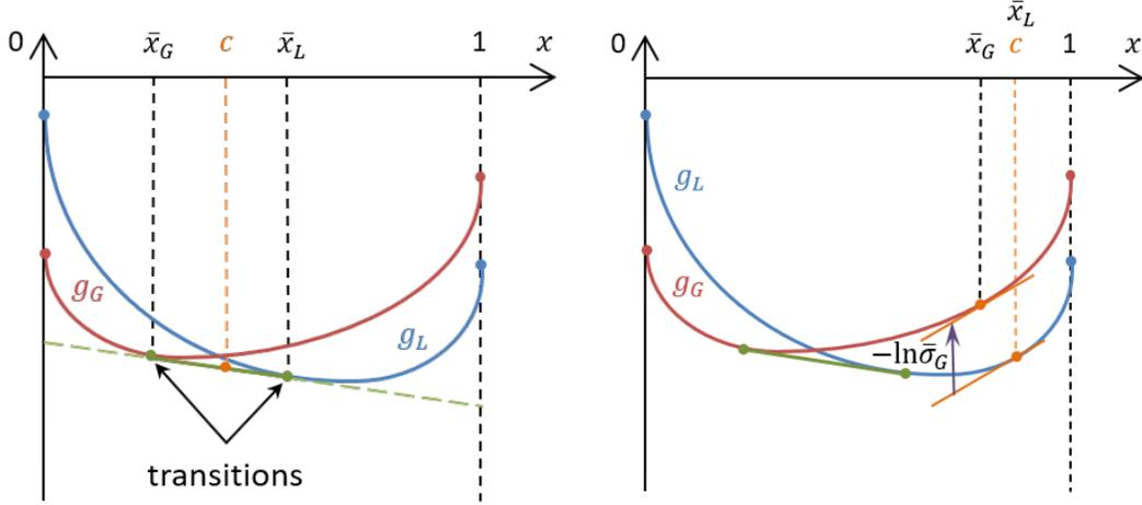
Figure 1: Gibbs' geometric construction for the phase equilibrium of a two-phase binary mixture. Left: two-phase solution. Right: single-phase solution.
