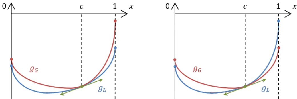
Figure 2: Azeotropic compositions for a two-phase two-component mixture.
