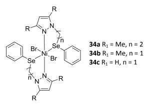
Figure 19. Selenium-functionalized pyrazole complexes
