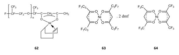
Figure 30. Perfluorinated Ni-complexes for FBS olefins oligomerization
