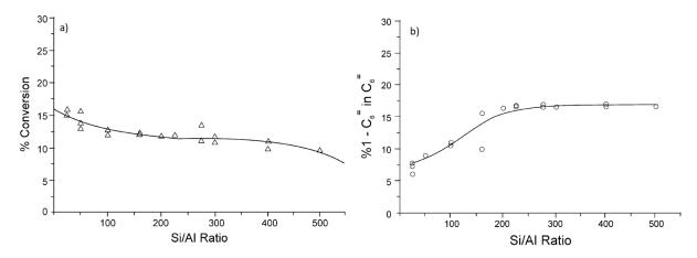
**Figure 40.** a) Ethene conversion and b) 1-Hexene selectivity as a function of Si/Al ratio of the support. T = 100  $\degree$ C, P = 1.5 MPa, MHSV = 4 h<sup>-1</sup>, and time-on-stream = 280 min. (Reproduced with permission from ref 281. Copyright 2003 Elsevier)
