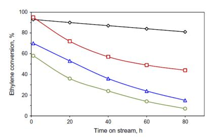
**Figure 44.** Activity profile of ( $\diamond$ ) Ni-AlSBA-15 outperforming ( $\Box$ ) Ni-MCM-41, ( $\Delta$ ) Ni-SiO<sub>2</sub>-Al<sub>2</sub>O<sub>3</sub> and ( $\circ$ ) Ni-Y. (Reproduced with permission from ref 334. Copyright 2015 Elsevier)
