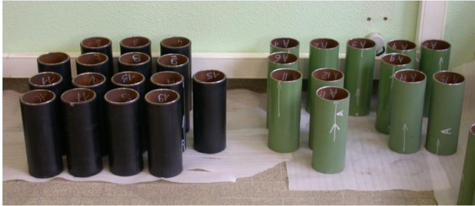
Figure 3 - 3-LPE tubes (on the left) and bi-layer tubes (on the right) as received
