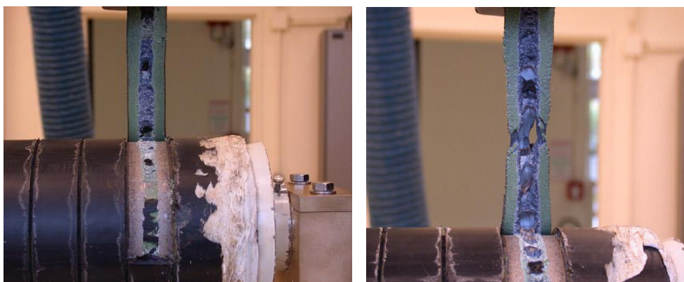
Figure 6 - Peeling of the B-3LPE coating aged 21 days in 3 % NaCl solution under -1,1 V vs. Ag/AgCl
