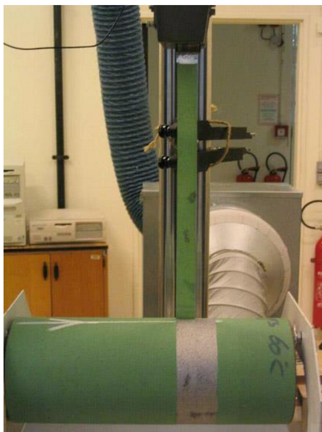
Figure 7 - Peeling of the bi-layer coating after a few weeks ageing at 60°C
