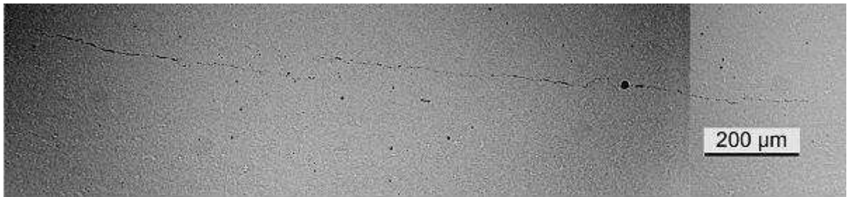
Figure 13: Metallographic observation of cracking in X70 SwS steel (L plan).
