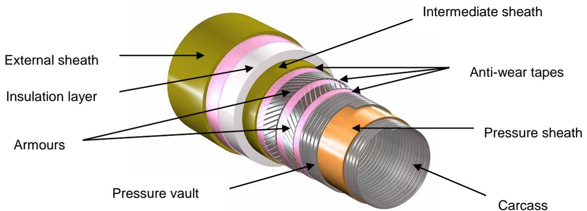
**Figure 1: Example of a flexible pipeline structure**
