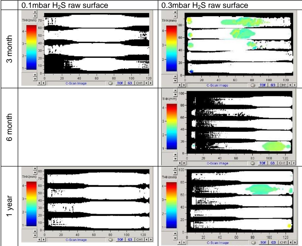
**Figure 4: Evolution of HIC extent on sweet steel (A) specimens exposed at ambient temperature and pressure in a 35 g/L NaCl solution saturated with 999.7 mbar CO<sub>2</sub> + 0.3 mbar H<sub>2</sub>S and with 999.9 mbar CO<sub>2</sub> + 0.1 mbar H<sub>2</sub>S .**
