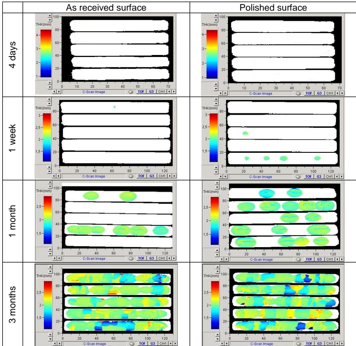
Figure 3: Evolution of HIC extent on sweet steel (A) specimens exposed at ambient temperature and pressure in a 35 g/L NaCl solution saturated with 997 mbar CO<sub>2</sub> + 3 mbar H<sub>2</sub>S and at pH 6.
