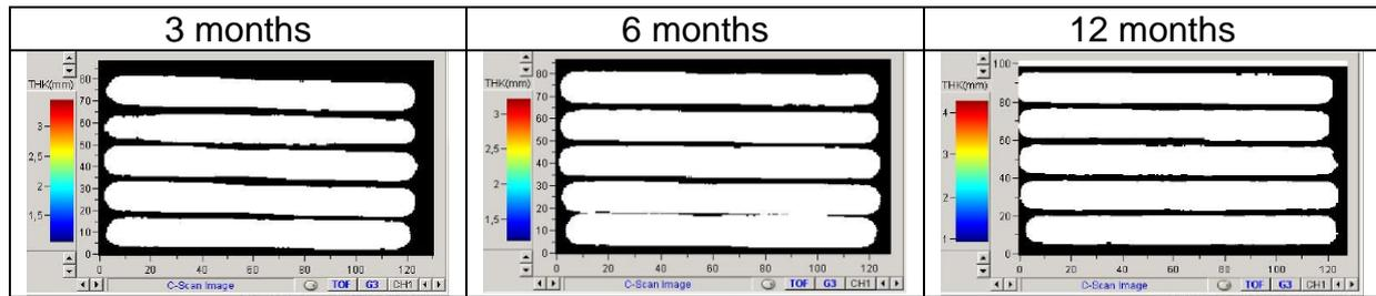
**Figure 5: HIC results on a mild sour high strength carbon steel grade tested at pH 5.5 under 1 mbar H<sub>2</sub>S for 3 months to 1 year**
