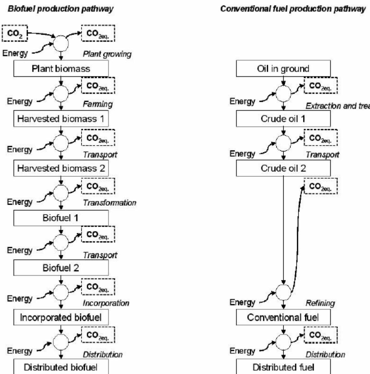
Figure 3: LCA scheme
