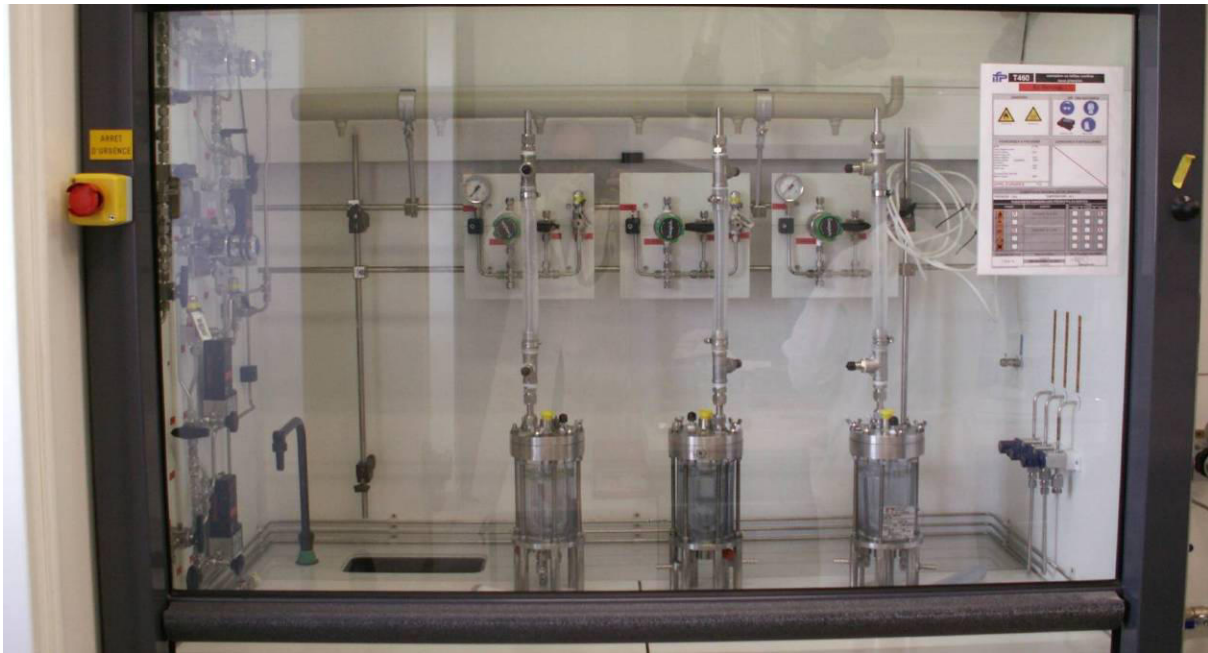
Figure 2: Experimental device for pH measurements in confined environments at pressure up to 10 bara
