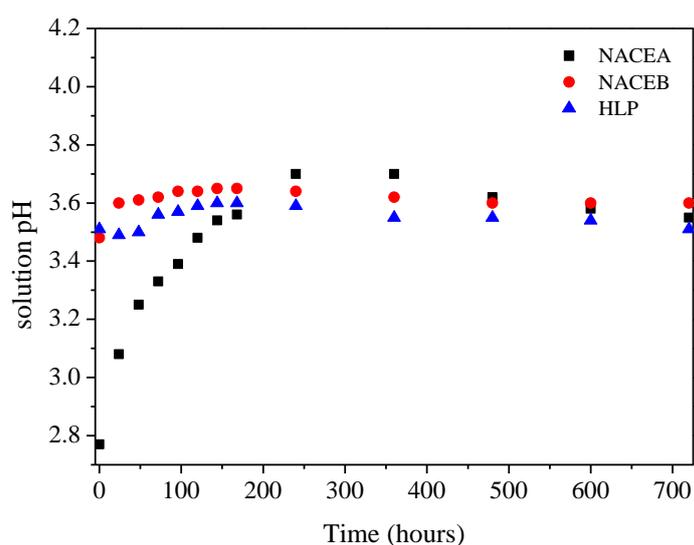
Fig 1: Evolution of test solution pH as a function of time over 720 h ( $T = 24^{\circ}\text{C}$ ,  $P_{\text{H}_2\text{S}} \sim 1 \text{ bar}$ ).
