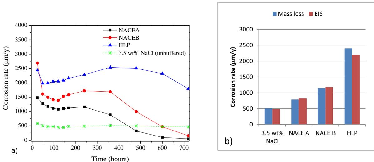
Fig. 2: Time evolution of the corrosion rate obtained from electrochemical measurements (a) and average corrosion rates determined from mass loss and electrochemical measurements (b) of X65 membrane exposed to buffer solutions at  $T = 24^{\circ}\text{C}$  under 1 bar  $\text{H}_2\text{S}$ .
