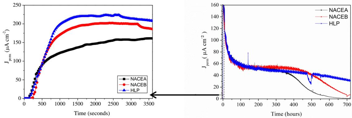
Fig 3: Hydrogen permeation across X65 membrane exposed to buffer solutions at  $T = 24^\circ\text{C}$  under 1 bar  $\text{H}_2\text{S}$ . The graph on the left shows the very initial peak ( $J_{\text{max}}$ ).
