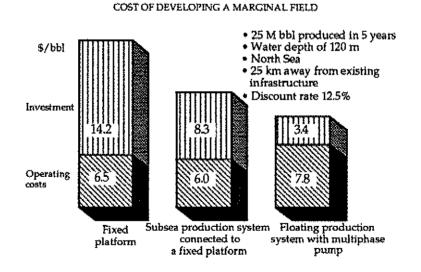
Lastly, new concepts combining subsea well heads with floating light production systems connected by flexible pipelines are making possible the economic development of marginal fields located in mature zones such as the Gulf of Mexico or the North Sea. Here again, there is an impressive potential for cost cutting, such as reducing investment by increasing operating costs, the latter having much less effect on the profitability of the project.
