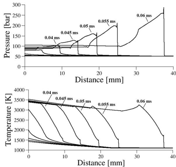
Fig. 9: Hot spot auto-ignition for case D ( $r_0 = 22.7$  mm,  $\Delta T_0 = 245.2$  K,  $\varepsilon = 16.9$ ,  $\xi = 5.4$ ,  $P_0 = 50$  bar,  $T_0 = 1100$  K,  $\phi = 1$ ,  $\tau_i = 0.286$  ms). Time sequence from 0.01 ms up to 0.06 ms.
