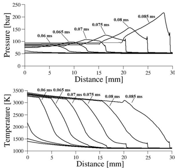
Fig. 8: Hot spot auto-ignition for case C ( $r_0 = 15.7$  mm,  $\Delta T_0 = 169.6$  K,  $\varepsilon = 11.1$ ,  $\xi = 8.7$ ,  $P_0 = 50$  bar,  $T_0 = 1100$  K,  $\phi = 1$ ,  $\tau_i = 0.286$  ms). Time sequence from 0.030 ms up to 0.085 ms.
