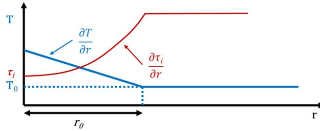
Fig. 3: Initial hot spot definition.
