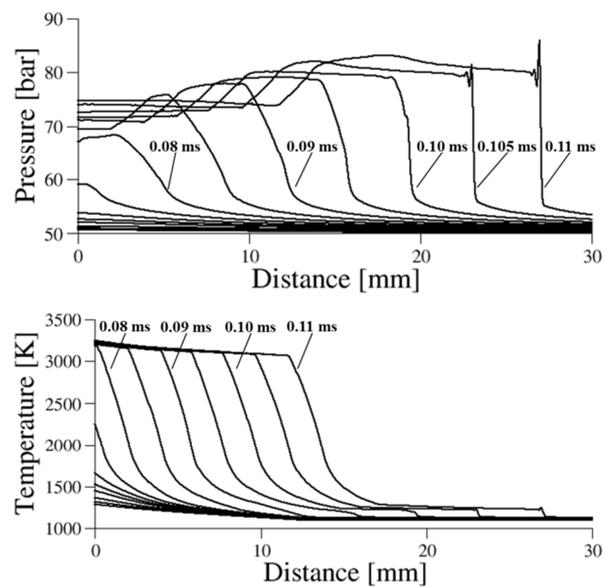
Fig. 7: Hot spot auto-ignition for case B ( $r_0 = 12.2$  mm,  $\Delta T_0 = 131.8$  K,  $\varepsilon = 7.9$ ,  $\xi = 10.7$ ,  $P_0 = 50$  bar,  $T_0 = 1100$  K,  $\phi = 1$ ,  $\tau_i = 0.286$  ms). Time sequence from 0.03 ms up to 0.11 ms.
