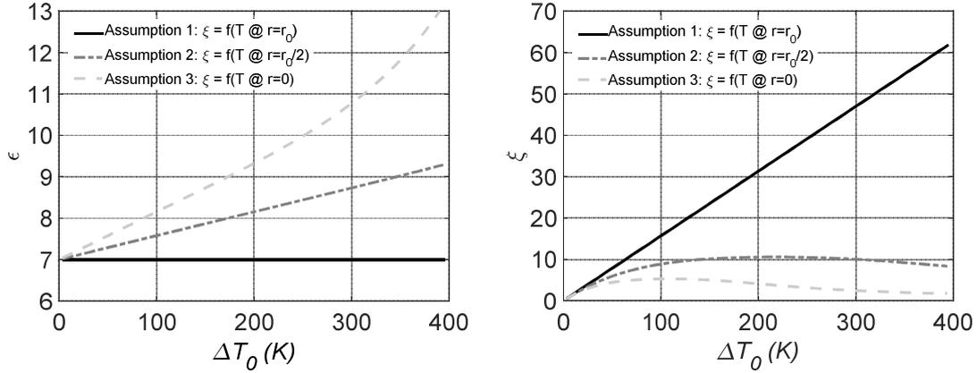
Fig. 4: Impact of the reference temperature on  $\varepsilon$  (top) and  $\xi$  (bottom) values as a function of  $\Delta T_0$  at the center of the hot spot ( $r_0 = 12.1$  mm,  $P_0 = 50$  bar,  $T_0 = 1100$  K,  $\phi = 1$ , no dilution).
