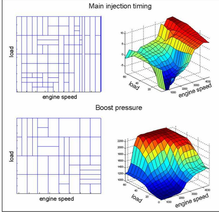
Figure 6: Examples of LoLiMoT parameterization of engine map. Left: patching of the domain. A local linear model is defined on each patch. Right: the resulting surfaces modeled by LoLiMoT for two different engine control parameters from given discrete reference maps.
