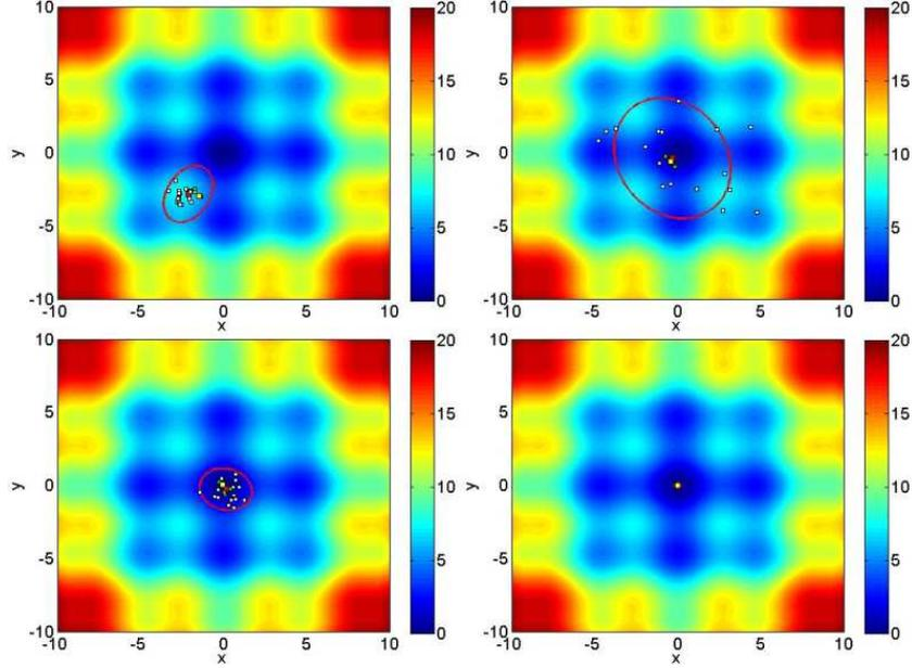
Figure 3: An application of CMA-ES method on the analytical function  $f(x, y) = \frac{x^2+y^2}{10} - \frac{1}{2}(\cos(\frac{2\pi}{5}x) + \cos(\frac{2\pi}{5}y)) + 3$ . From top left to bottom right, the population at iterations 1, 5, 8 and 20 are represented. The ellipse represents the 95%-isovalue of the Gaussian probability density of the mutation operator with the adaptive covariance matrix.
