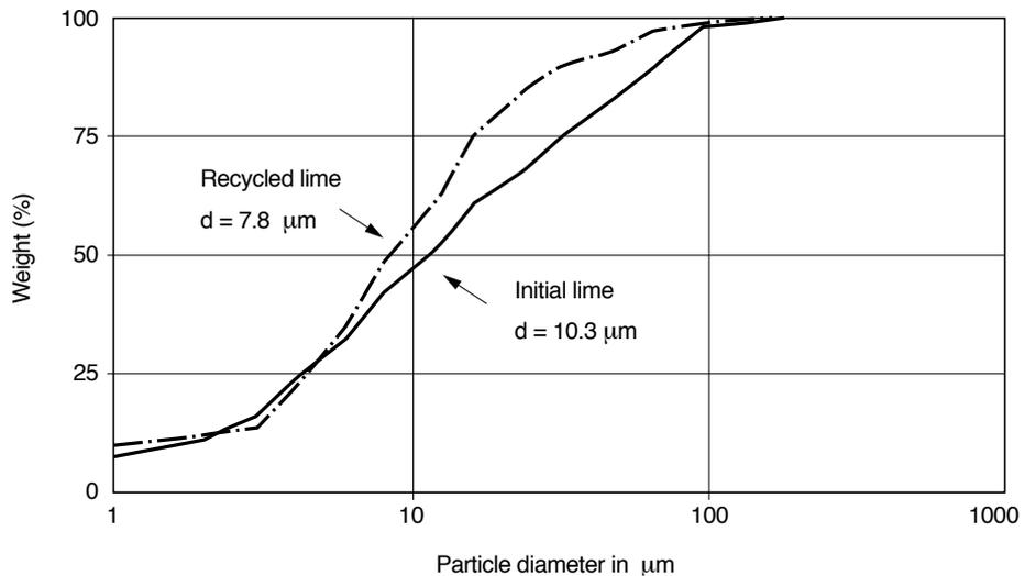
granulometry ( $d = 7.8 \mu\text{m}$ ) than that of the one initially mixed with sand ( $d = 10.3 \mu\text{m}$ ). This means that only the thinner particles are transported by the gas stream. This is in fact fairly coherent since such particles have smaller free fall velocities compared to the one remaining in the bed.
