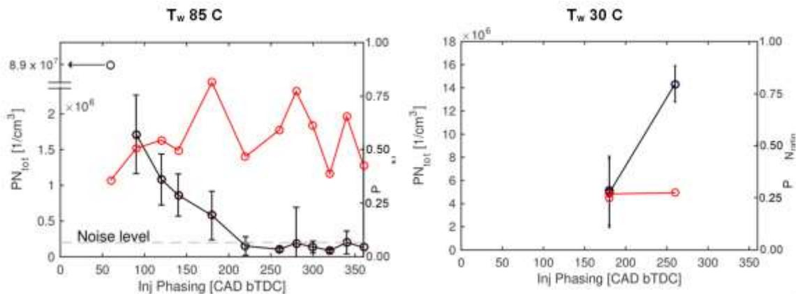
Fig. 8: Effect of injection phasing on  $PN_{tot}$ , (in black, on the left y-axis) and  $PN_{ratio}$ , (in red, on the right y-axis). The standard deviation is presented together with the  $PN_{tot}$  values.
