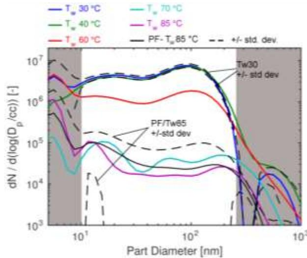
Fig. 4: Effect of  $T_w$  on particulate emissions. The part of the spectrum not considered for the analysis is indicated by the gray areas. The measurement obtained in port-fuel injection mode is plotted in solid black line for reference.
