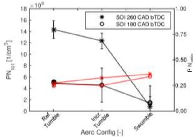
Fig. 11: Effect of in-cylinder aerodynamics on  $PN_{tot}$ , (in black, on the left y-axis) and  $PN_{ratio}$ , (in red, on the right y-axis). The standard deviation is presented together with the  $PN_{tot}$  values.  $T_w = 30\text{ C}$ .
