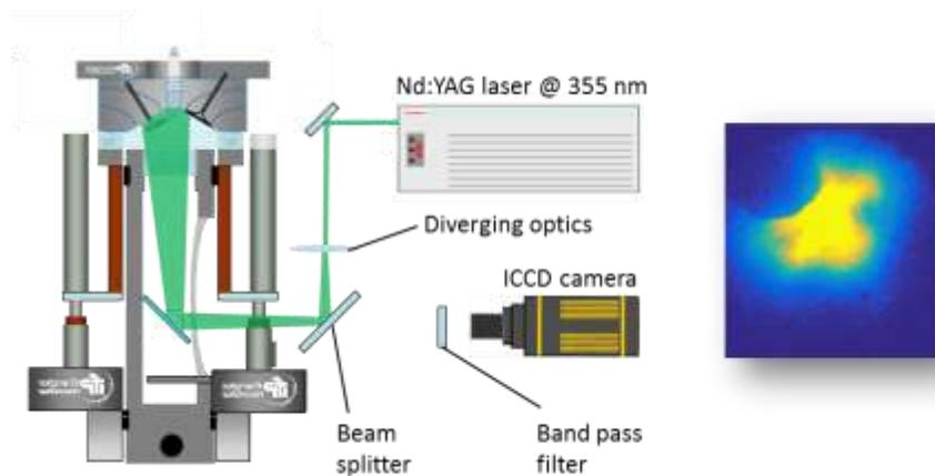
Fig. 3: Optical layout for liquid fuel film visualization.
