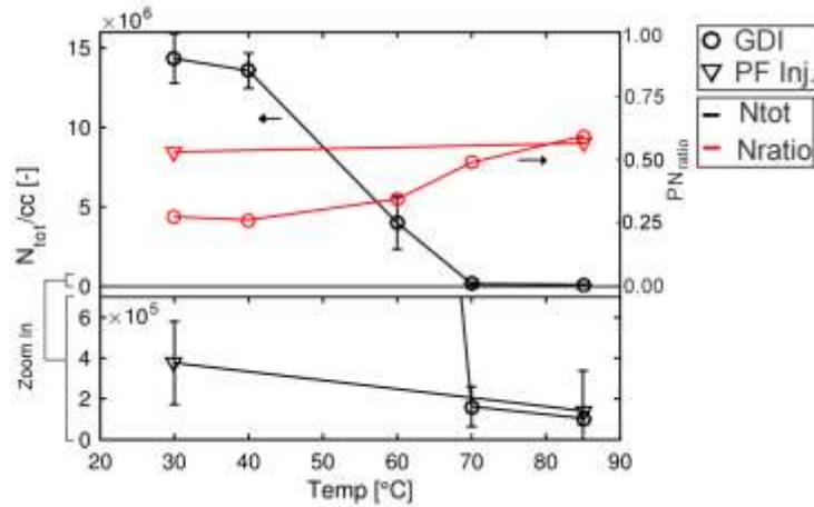
Fig. 5: Effect of  $T_w$  on  $PN_{tot}$  , (in black, on the left y-axis) and  $PN_{ratio}$  , (in red, on the right y-axis). The standard deviation is presented together with the  $PN_{tot}$  values. For GDI cases, SOI 260 CAD bTDC.
