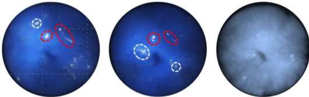
Fig. 6: Broadband color images for different engine temperatures taken at 15 CAD aTDC.  $T_w$  30 °C (left),  $T_w$  60 °C (center) and  $T_w$  85 °C (right). Soot formed in pool fires mode can be observed in the images (red circles).
