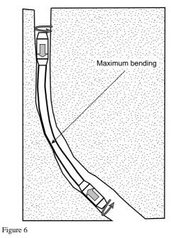
Maximum bending in compression drillpipe.
