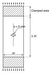
Figure 22 Central crack small-size specimen (as per [6]).
