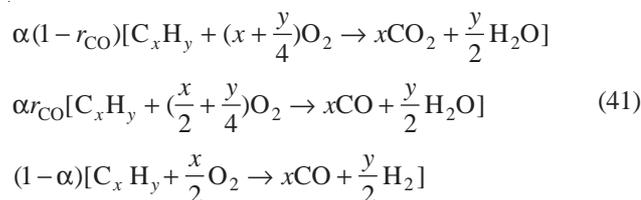
The coefficient  $\alpha$  is defined by the local equivalence ratio:
