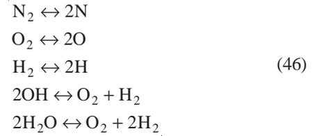
These equations can be reduced to one polynomial equation (6<sup>th</sup> degree). This equation is then solved using a Newton method, which is straightforward with a polynomial expression.
