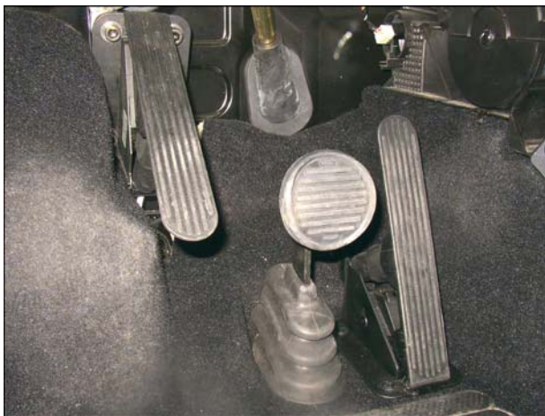
Picture 3 Added clutch pedal on the left side.
