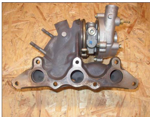
Picture 1 Exhaust manifold.
