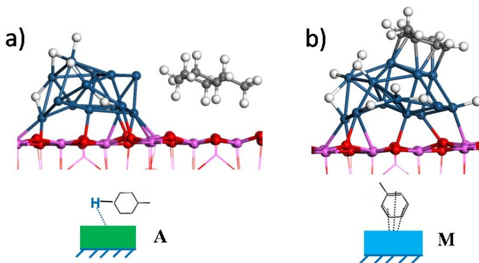
**Figure 5. a) Adsorption mode of (A) methyl-cyclohexane and b) of (M) toluene on  $\text{Pt}_{13}\text{H}_6/\gamma\text{-Al}_2\text{O}_3$ . Color legend: aluminum (pink balls), oxygen (red balls), platinum (dark blue balls), carbon (dark grey balls), hydrogen (white balls)**
