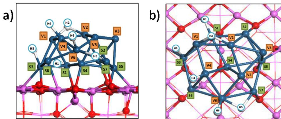
**Figure 1. Molecular structure of the starting model of Pt<sub>13</sub>/γ-Al<sub>2</sub>O<sub>3</sub> (100) with 6 adsorbed hydrogen atoms. a) side view, b) top view. Pt atoms labelled with letter “S” are located at the alumina surface, Pt atoms labelled with letter “V” are in contact with vacuum. Color legend: aluminum (pink balls), oxygen (red balls), platinum (dark blue balls), hydrogen (white balls)**
