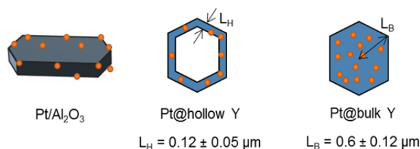
Scheme 1. Schematic representation of the various materials and their corresponding characteristic length.
