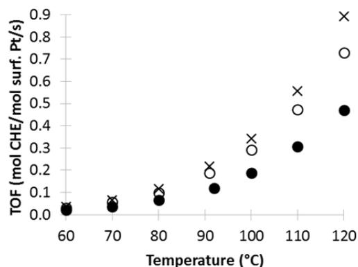
**Figure 2.** Cyclohexene apparent turn over frequencies (TOF) measured over (x) Pt/Al<sub>2</sub>O<sub>3</sub>, (●) Pt@bulk Y and (○) Pt@hollow Y. Feed = 3.3 % in H<sub>2</sub>, total flow = 20 mL min<sup>-1</sup>.
