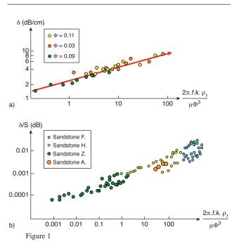
Relationship between attenuation and petro-physical parameters (after Morlier and Sarda, 1971). Laboratory measurements on cores with a) constant specific surface and b) variable specific surface.
