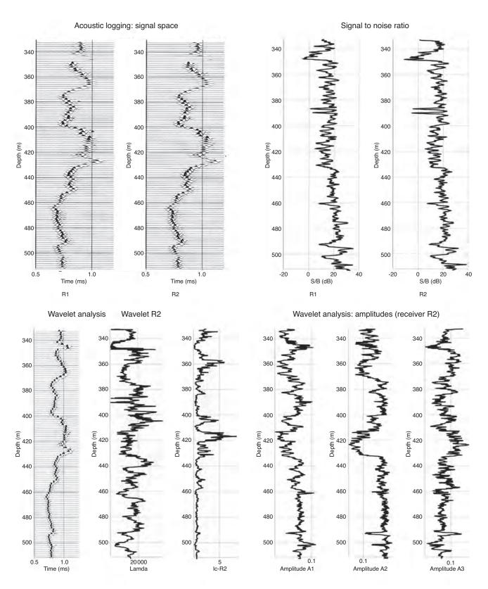
Analysis of refracted waves in acoustic logging by Singular Value Decomposition (SVD).
