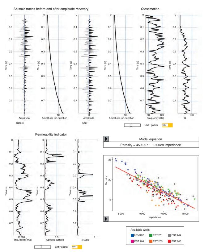
Seismic analysis at CMP 600.
