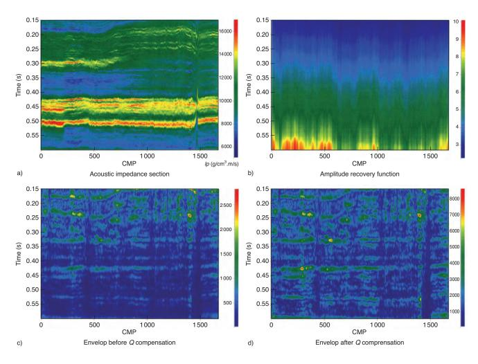
Seismic analysis: amplitude recovery. a) Acoustic impedance seismic section. b) Amplitude recovery function section.
