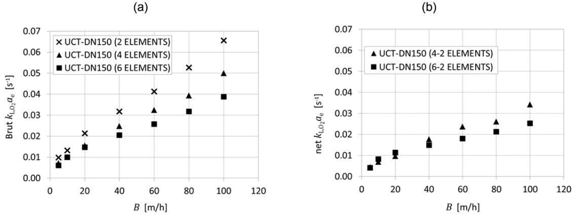
Figure 3.  $k_L a_e$  measured with original wall wipers only for different bed heights in the UCTP-DN150 column at  $F_s = 0.02 \sqrt{\text{Pa}}$  for (a) brut values and (b) net values.
