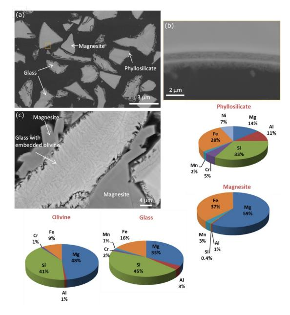
943 **S8.** SEM images of the ionically polished sections of experimental product at T = 523 K and P =944 30 MPa showing euhedral magnesite crystals and secondary phyllosilicates. (b) a magnified view 945 of phyllosilicate (c) SEM image of a polished section of the products showing magnesite with 946 zoning. The chemical composition obtained by SEM EDX analysis is shown in pie charts.
