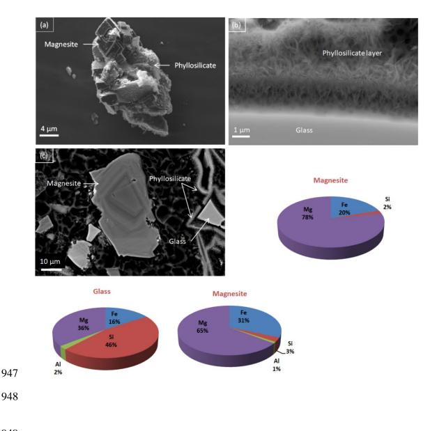
950 S9. SEM images of the ionically polished sections of experimental product at T = 573 K and P =951 30 MPa, showing anhedral magnesite formed around glass, and heavily altered glass with thick 952 layers of phyllosilicate.
