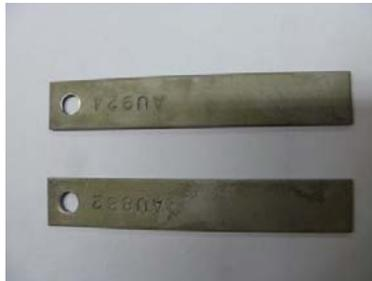
Fig. 12 : Stripper inlet carbon steel coupons recovered at the end of DMX long-run test (~1500h)
