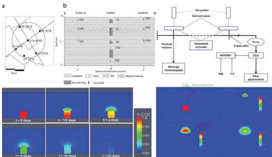
Fig. 1. (top) Map of gas probes implementation on the experimental site and schematic representation of the gas analyses device; (bottom) Numerical simulations of CO<sub>2</sub> leakage from the cavity (left) and from the CK4 point in the well (right).
