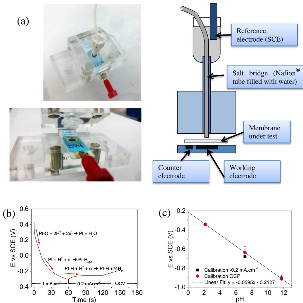
**Figure 2. Raw data for DHE measurement of several membranes.**
