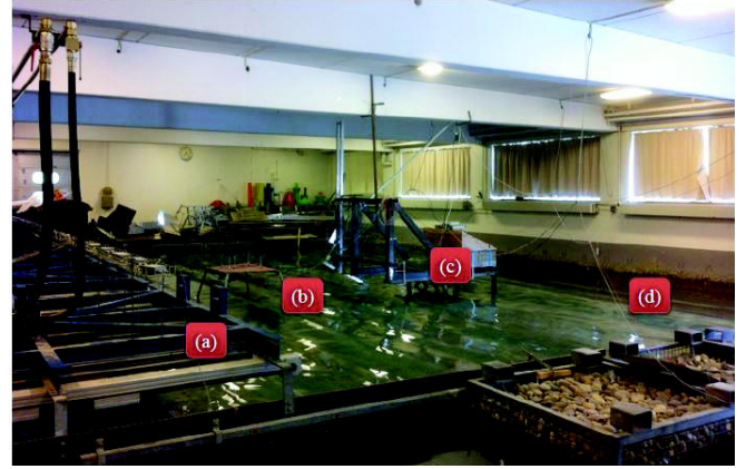
Fig. 4. Experimental setup at AAU. The waves are generated by the wave generation system (a) and the wave elevation is measured by a series of wave gauges (b). The waves then reach the WEC laboratory model, where the wave energy absorption takes place (c). Finally, they reach the artificial beach where the termination takes place by a scattering process (d).
