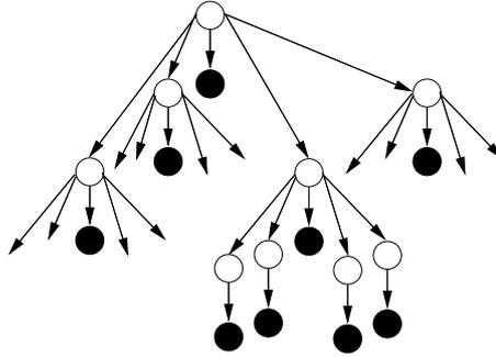
Fig. 1. Diagram of a hidden Markov tree in a quad-tree. White dots represent hidden states with arrows as dependencies, black dots the transformed coefficients. The black dot on the top represents a parent coefficient with its four children.
