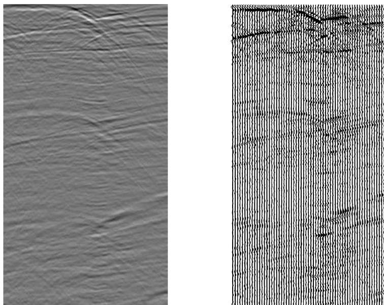
Fig. 8. Example of stacked seismic data in classical image form (left) and with a wiggle plot (right).
