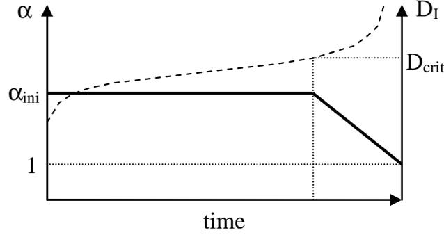
**Fig. 3** Evolution of parameter  $\alpha$  with damage
