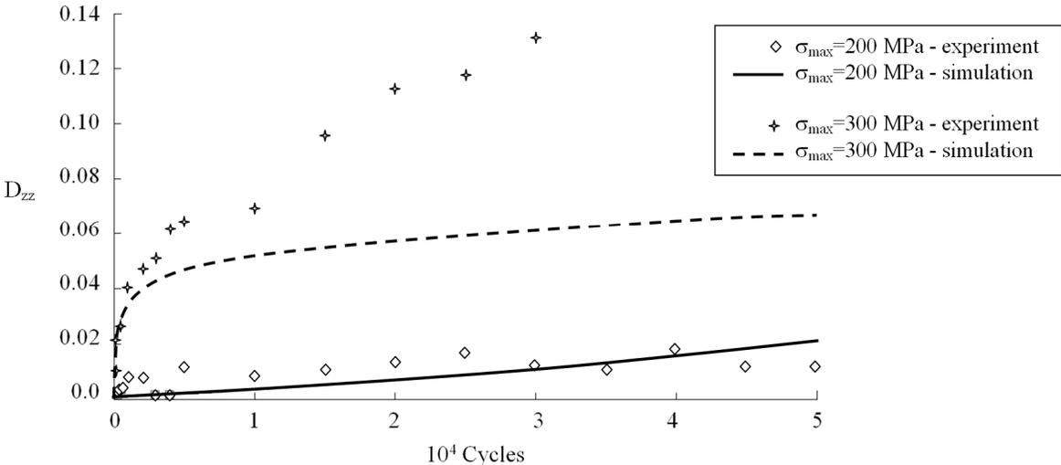
**Fig. 7** Comparison of the damage evolution resulting from the model and fatigue tests at different loadings -  $R=0.1$ ,  $f=2$  Hz - on  $[\pm\theta/\pm\phi]$  lay-up
