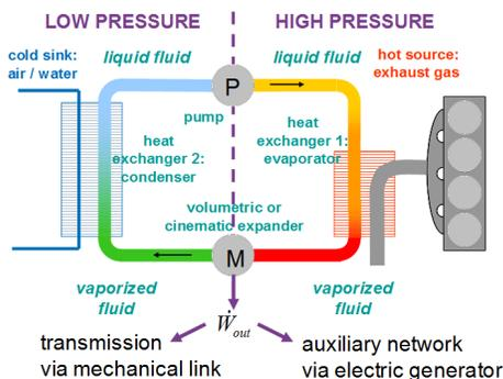
Fig. 1. Rankine WHR system layout for automotive applications
