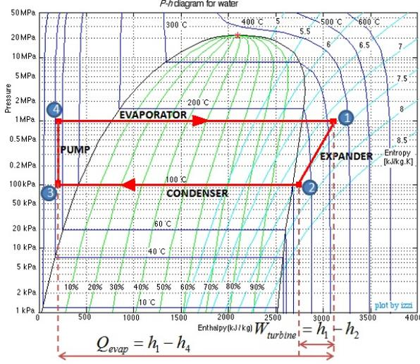
Fig. 4. Rankine cycle on water  $p-h$  diagram
