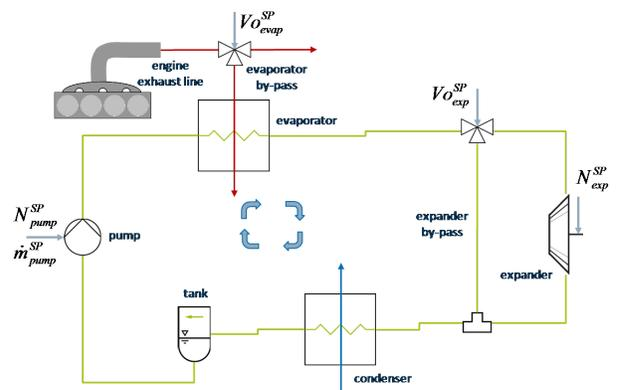
Fig. 2. Layout of Rankine steam process under consideration
