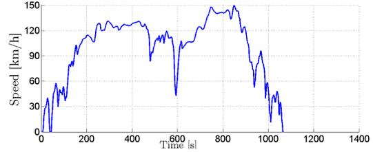
Fig. 8. Speed profile for the Artemis Motorway Cycle
