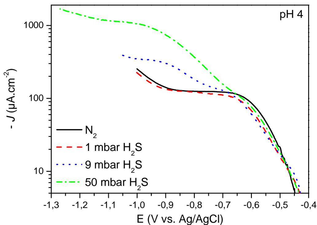
Figure 2: Stationary cathodic polarization curves measured with a RDE at 180 rpm in de-aerated solution containing different amount of H<sub>2</sub>S at pH 4
