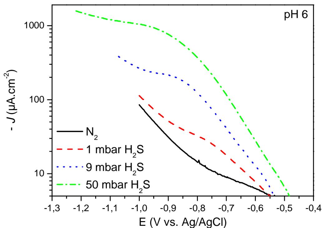
Figure 3: Stationary cathodic polarization curves measured with a RDE at 180 rpm in de-aerated solution containing different amount of H<sub>2</sub>S at pH 6
