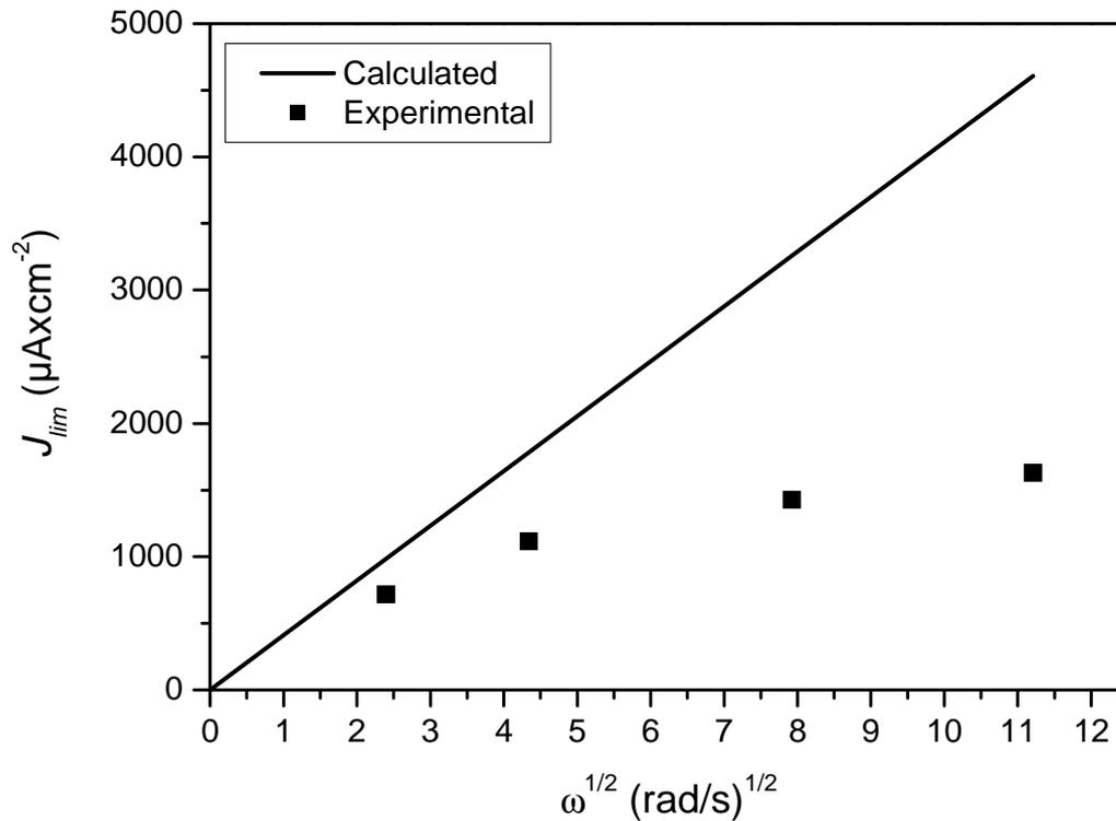
**Figure 5: Evolution of the limiting cathodic current with the rotation speed of the electrode in de-aerated solution containing at pH 6 with 50 mbar H<sub>2</sub>S**
