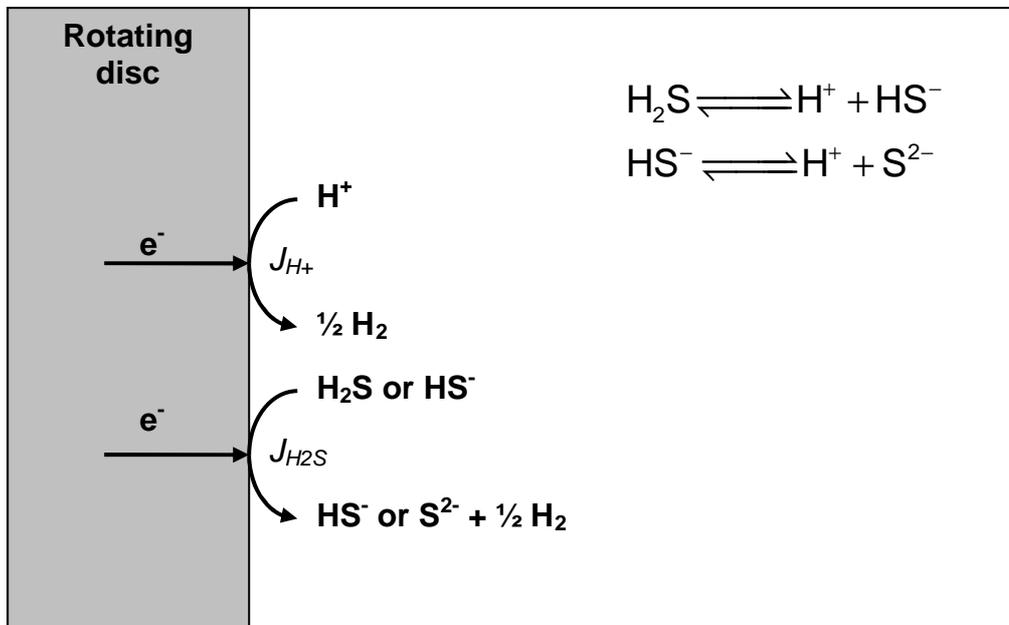
Figure 7: Scheme of the system describing cathodic reactions in acid water containing dissolved H<sub>2</sub>S
