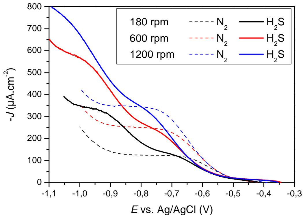
Figure 1 : Stationary cathodic polarization curves measured with a RDE at pH 4 in  $\text{N}_2$  purged solution or in  $\text{H}_2\text{S}$  saturated (9 mbar) solution
