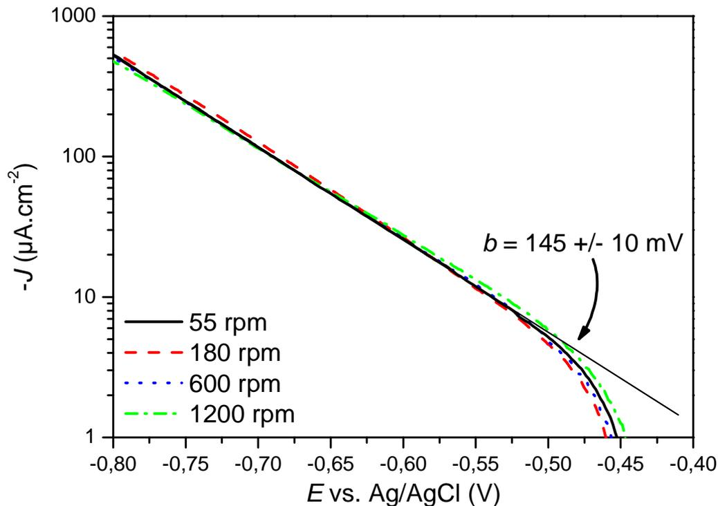
Figure 6: Tafel plots of the kinetic part of the cathodic current ( $J_k$ ) in pH 6 solution saturated with 50 mbar H<sub>2</sub>S
