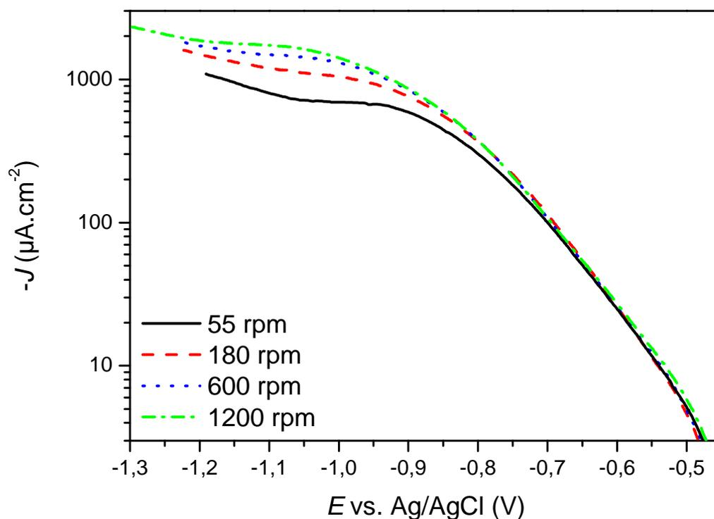
Figure 4: Experimental stationary cathodic polarization curves measured with a RDE at different rotation speed in de-aerated solution containing at pH 6 with 50 mbar H<sub>2</sub>S
