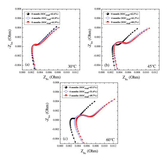
Fig. 5. Impedance spectra measured at  $25^{\circ}$ C and  $SOC_{nom,ck} = 60\%$  for (a) a cell aged at  $30^{\circ}$ C and  $SOC_{nom} = 100\%$ , (b) a cell aged at  $45^{\circ}$ C and  $SOC_{nom} = 100\%$ , (c) a cell aged at  $60^{\circ}$ C and  $SOC_{nom} = 100\%$ . The real SOC values corresponding to each spectrum are provided in the plot legends.
