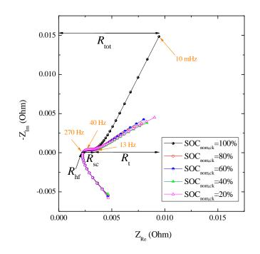
Fig. 4. Impedance spectra of the fresh cell measured at 25°C and at different nominal checkup SOCs (20%, 40%, 60%, 80%, and 100%).
