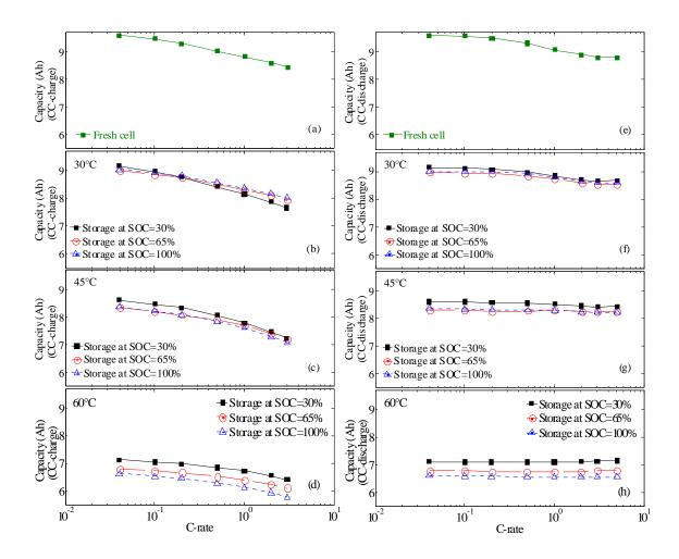
Fig. 3. Rate capability of both fresh and aged cells under different storage conditions of temperature and nominal SOCs, measured at 25°C before taking the cells apart. (a) to (d) Rate capability on charge; (e) to (h) Rate capability on discharge.
