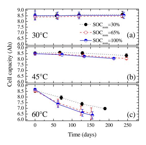
Fig. 2. Discharge capacities measured at  $1C_{nom}$  and  $25^{\circ}C$  for the 27 cells under different storage conditions of temperature and SOC.
