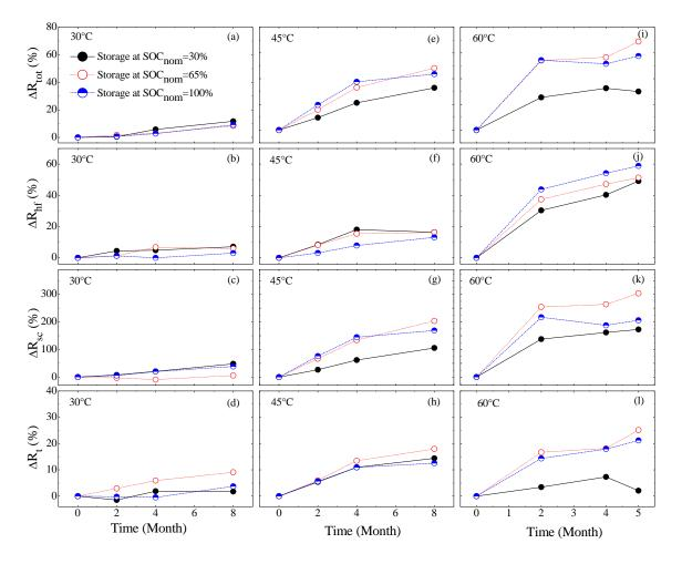
Fig. 6. Evolution of the total resistance  $R_{tot}$ , the ohmic resistance  $R_{hf}$ , the semicircle resistance  $R_{sc}$ , and the tail resistance  $R_t$  derived from the impedance spectra of the cells at 25°C and  $SOC_{nom,ck} = 60\%$ .
