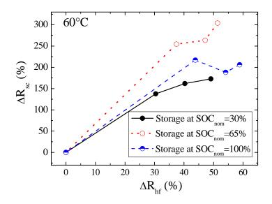
Fig. 7. Correlation plot of semicircle and high-frequency resistances for the cells aged at 60 °C and different nominal SOCs. The values were derived from the impedance spectra of the cells at  $25^{\circ}$ C and SOC<sub>nom,ck</sub> = 60%.
