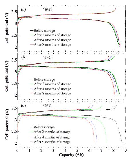
Fig. 1. Charge/discharge profiles measured at  $1C_{nom}$  and  $25^{\circ}C$  for cells under storage at SOC<sub>nom</sub>=100% and at temperature (a) 30°C, (b) 45°C, and (c) 60°C.
