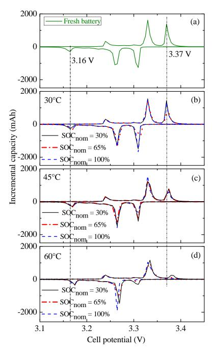
Fig. 9. Incremental capacity plot against cell potential derived from the PITT measurements at 25°C that are reported in Fig. 8.
